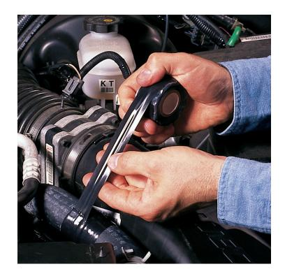
Silicone tape is available in numerous colors, so finding a color to wrap around your outdoor equipment is easy. Wrapping silicone tape around these parts protects the metal from the elements, prevents the start or spread of rust, and if you purchase more than one color, allows you to quickly identify equipment.
